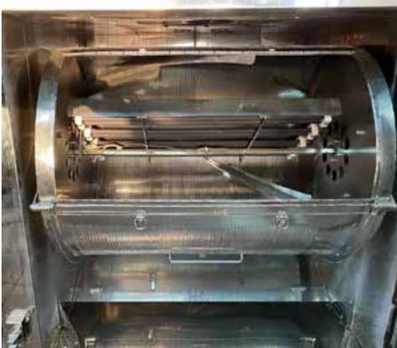
steel cylinder that slowly rotates. So the oven has normal electrical heating elements to maintain a constant atmospheric temperature. And the infrared elements are a supplemental heat source that emit infrared waves, which are particularly effective in penetrating the leaves, resulting in a significantly more uniform effect.
